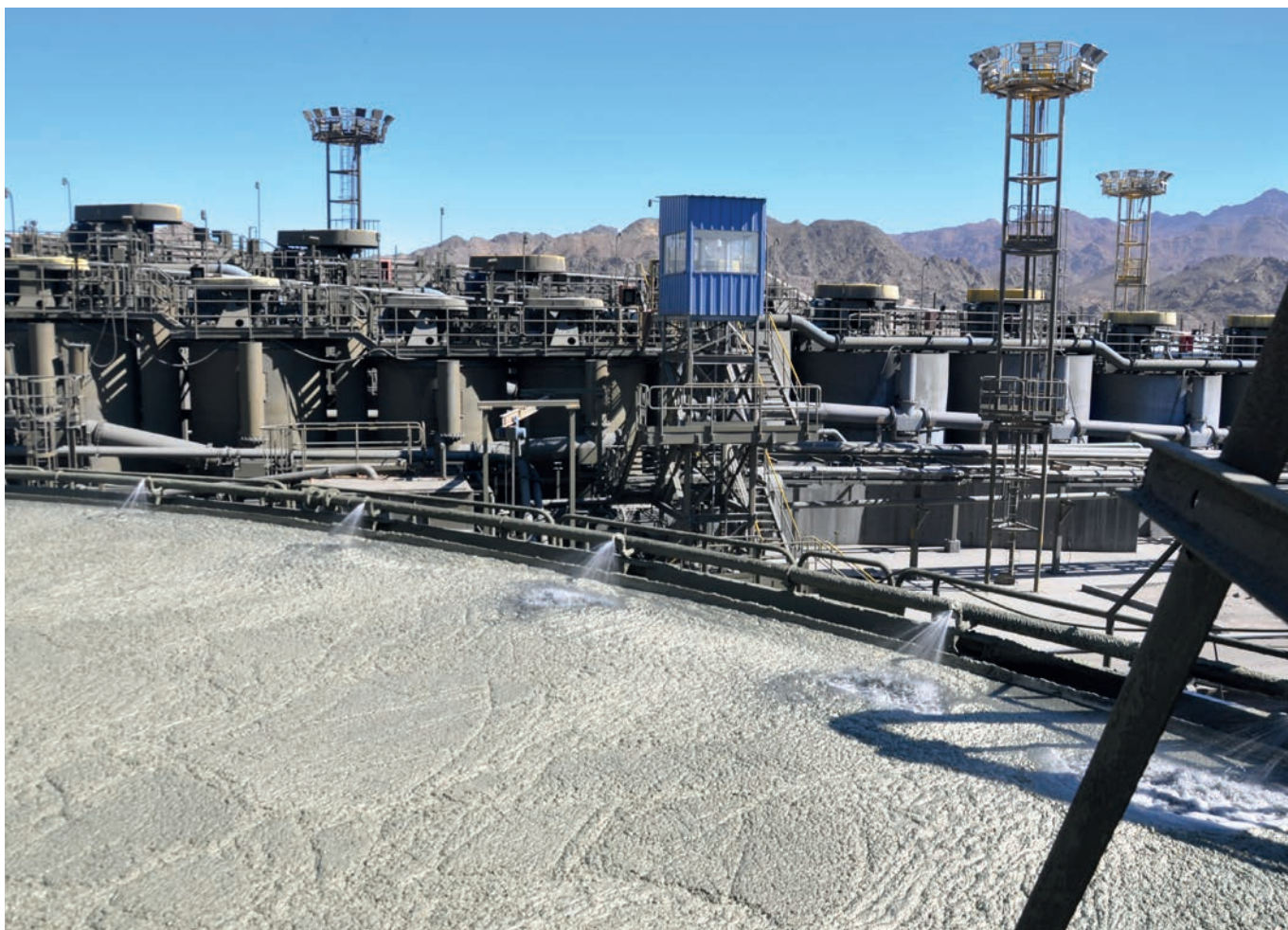
Concentrate thickeners are used to obtain 65% solids before concentrate is pumped through the slurry pipeline.
