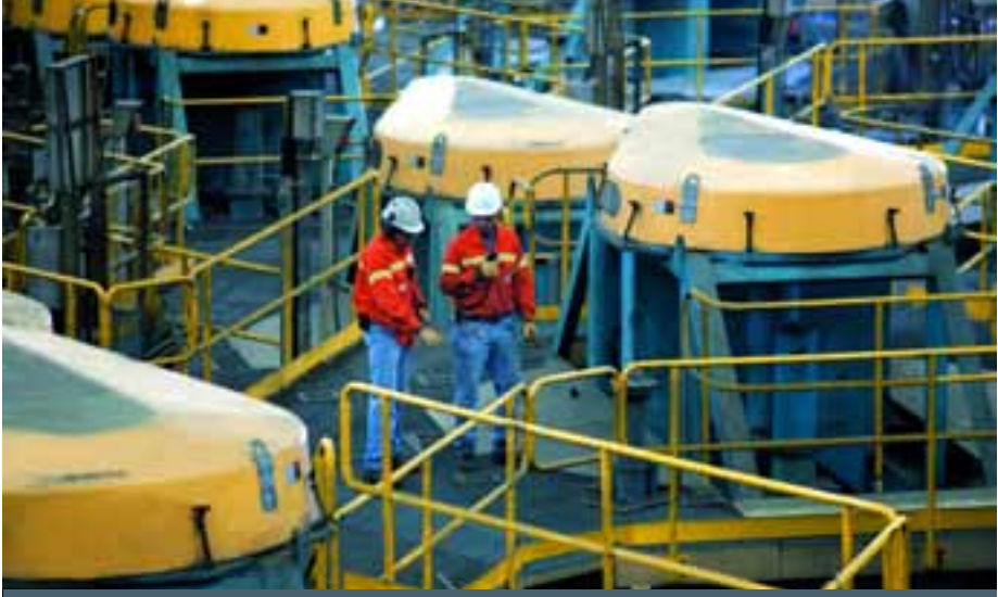
Concentrator maintenance operators, Alfredo Brizuela and Fulgencio Marcelo Colqui, are measuring air in flotation cells.
