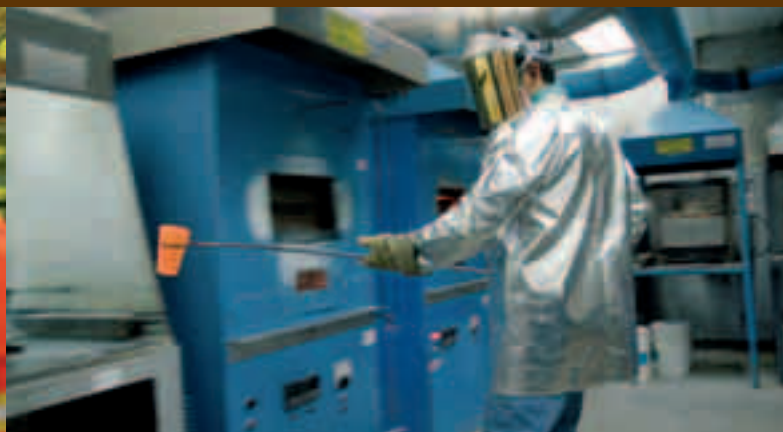
Chemical assayer Eduardo Robledo smelting concentrate samples
