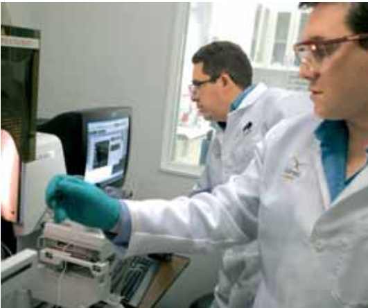
Juan G. Pani and Luis Cointte determining metal concentration through the atomic absorption process at Minera Alumbra's lab.
