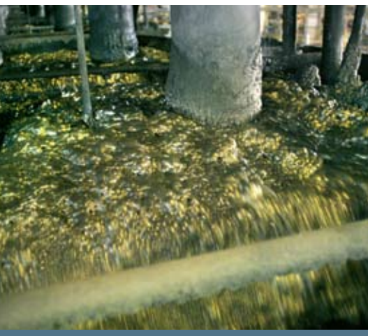
Concentrate is recovered through a flotation process.
