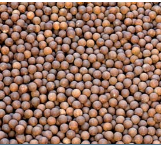
Steel balls being fed into the SAG mills to reduce rock size. 5.5 inch balls weigh 12 kg.
