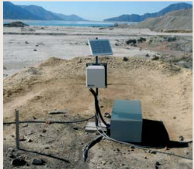
Capping and cover systems have sensors that measure humidity, pressure and temperature and this data is recorded to improve the designs to be implemented.
