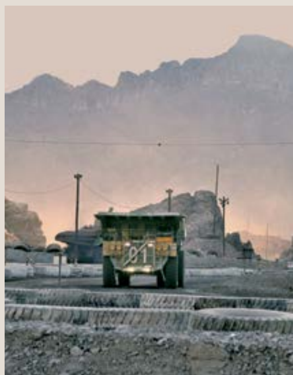
Heavy equipment can carry up to 220 tonnes of rock.
